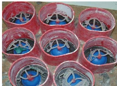
Figure 25. Prepared for investing. Note that there is no refractory model and therefore no "flash".
