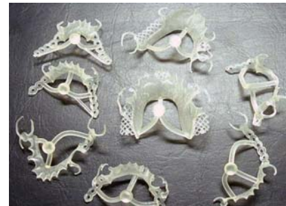
Figure 24. Frames with support wax removed, shown here with clear prototype resin.
