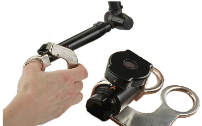
Scissors snap-on end effector
