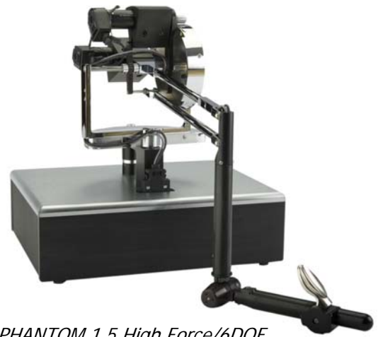
PHANTOM 1.5 High Force/6DOF with pinch end effector and palm seat
