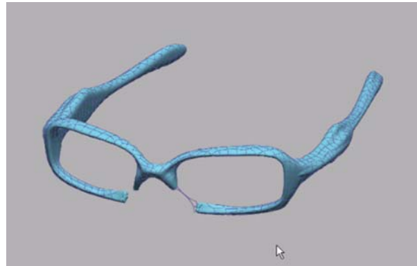
Incomplete auto surface result due to problem areas
