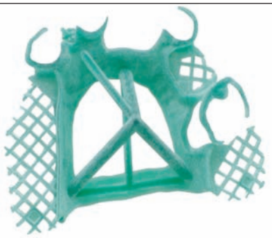
3-D printed resin pattern from the SensAble system.
