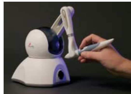
The Phantom Omni Haptic Controller hardware, used with ClayTools, mimics the physical properties of clay by creating resistance.
