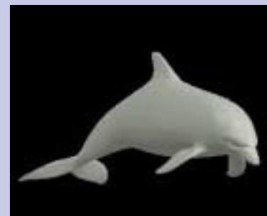
The finished model. In the custom-setting, the finest details have been added, the surfaces smoothed and lines refined. This digital model is ready to be exported as an STL file to a rapid prototyping machine, or to a NURB-surfacing package for importing into a 3D design or CAD package.
