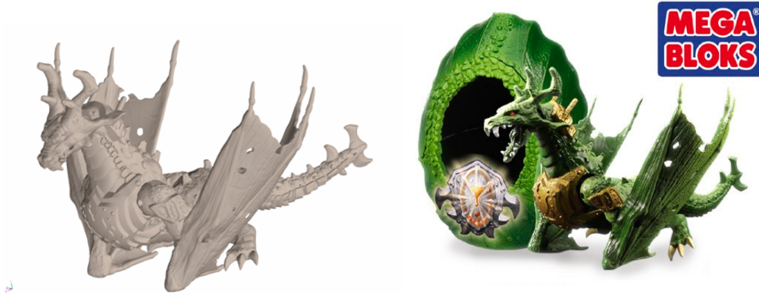
Design of a MEGA BLOKS Dragon in FreeForm (left) and the finished Serpentorch from the Dragons ™ collection (right)
