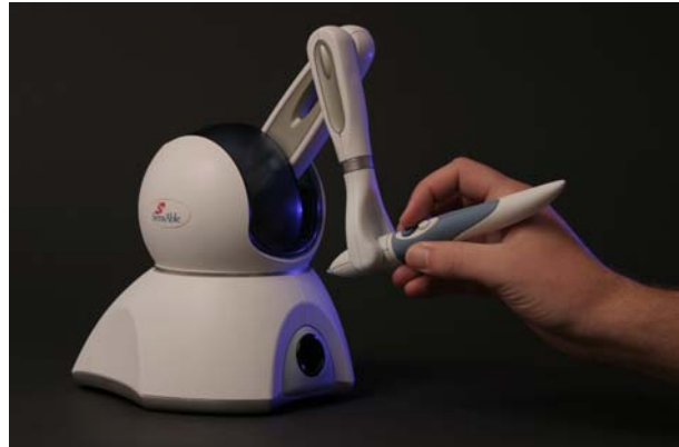
The FreeForm Concept system includes the PHANTOM® Omni™ haptic device which allows designers to use their sense of touch to model and apply paint, images, and other details.
